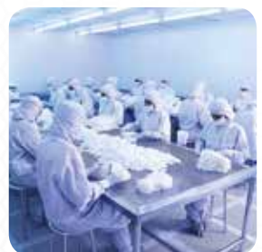
► Packing class in class 100 cleanroom
